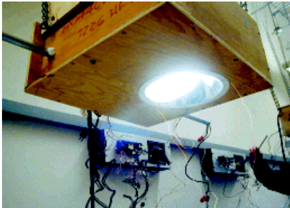
Photo 1. During UL 1598 luminaire tests, temperatures are measured by means of thermocouples and suitable indicating devices.
