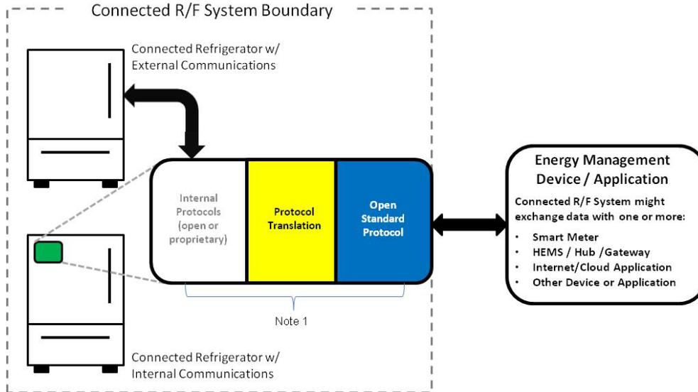
*Note 1: Communication device(s), link(s) and/or processing that enables open standards-based communication between the Connected R/F System and Energy Management Device/Application(s). These elements could be within the base appliance, and/or an external communication module, a hub/gateway, or in the Internet/cloud.*
