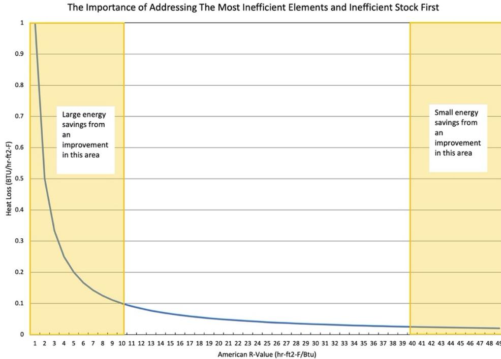
Figure 1. R-value is a counterintuitive unit of measure, not all R-values are the same, changes in R-value at the low end of the spectrum results in significant changes in heat loss/gain while even large changes in R-value at the high end of the spectrum nets only small changes in heat loss/gain. (PNNL 2020).
