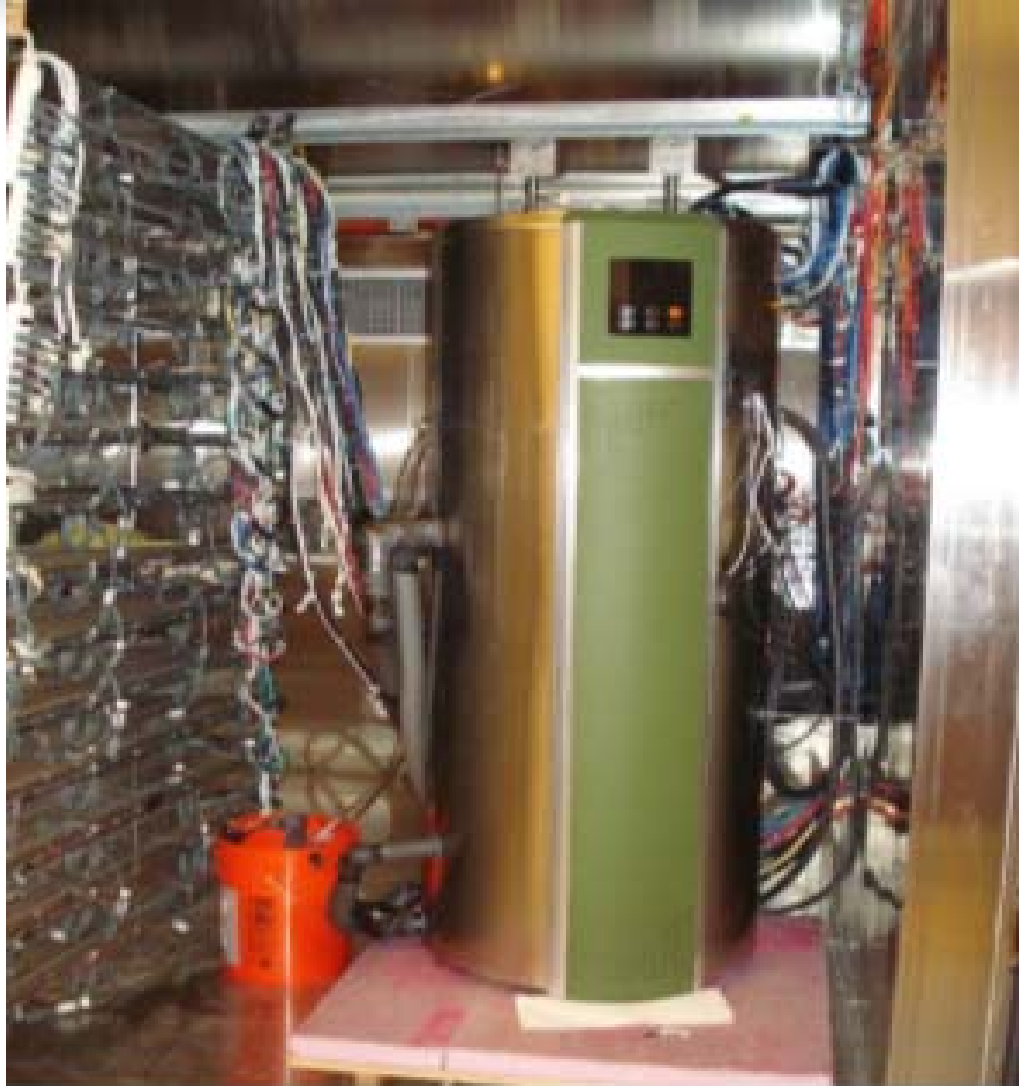
Air Generate in a Thermal Chamber
