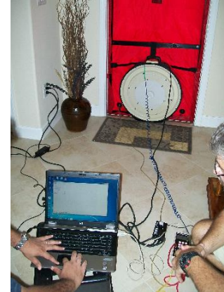
Enclosure and duct leakage: Delta Q.
