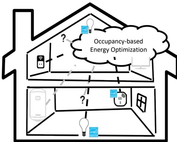
**Figure 1: Simple illustration of the basic elements of an ENERGY STAR Smart Home Energy Management System** (consisting of required minimum devices shown with black dotted lines, optional devices in gray, and the core service capability, occupancy-based energy optimization)
