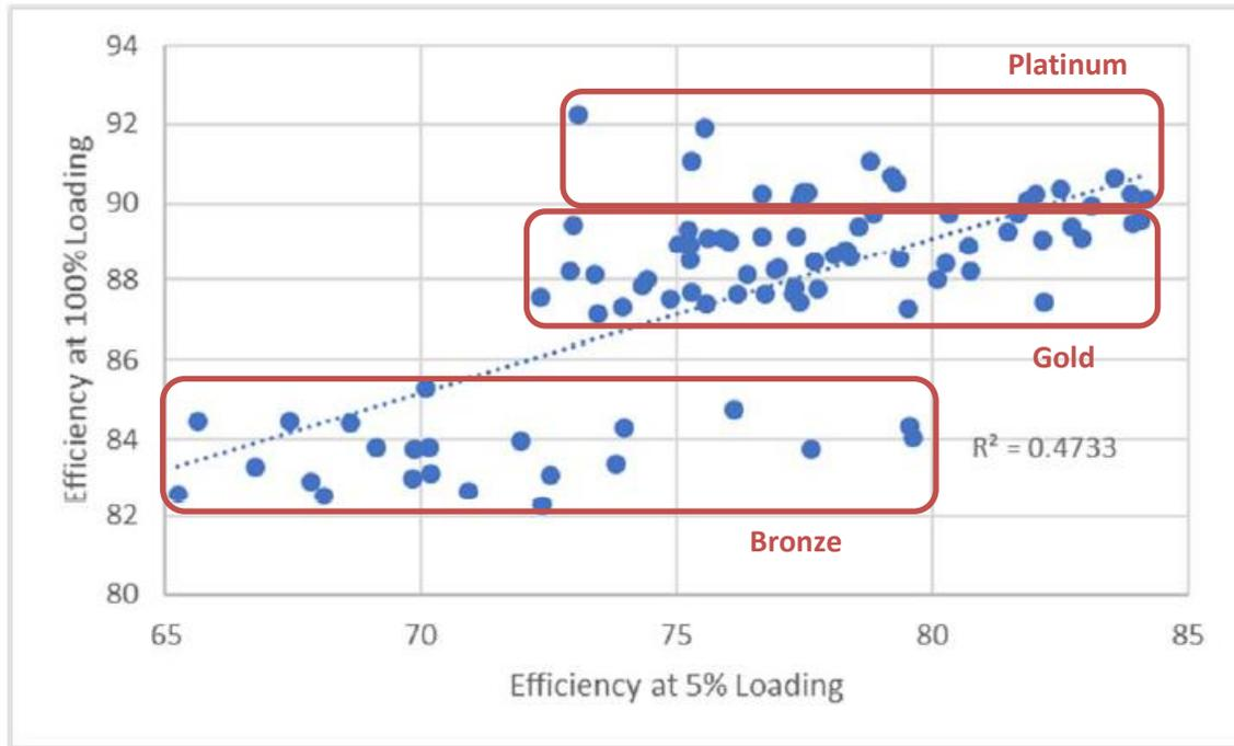
Figure 3. Efficiency at 5% Loading versus Efficiency at 100% Loading.
