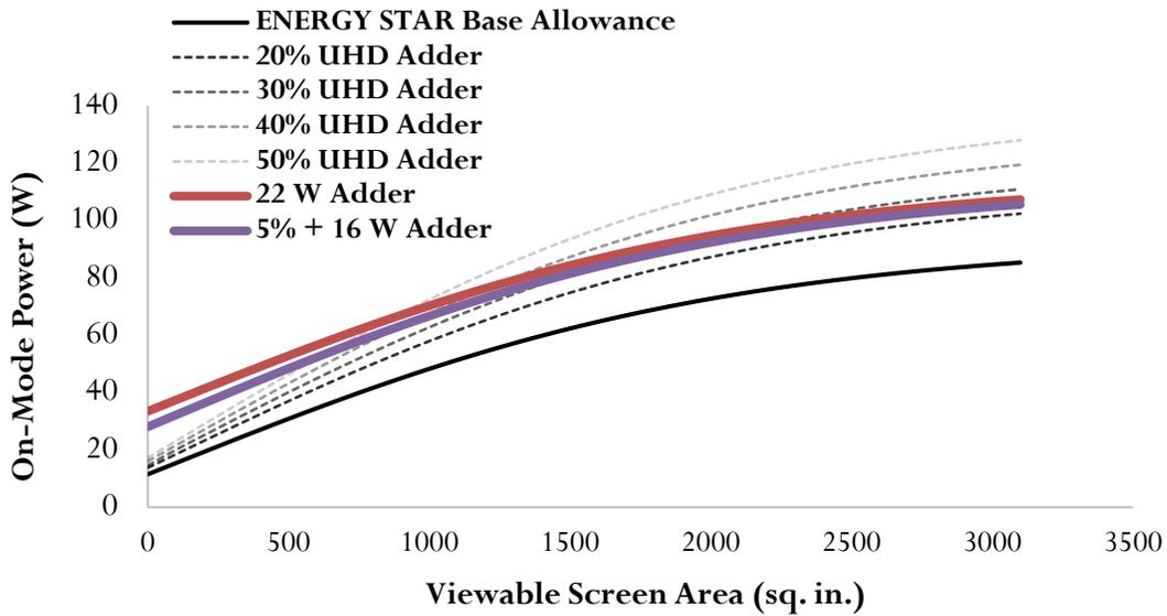
Figure 2. On-mode power vs viewable screen area for ENERGY STAR v7 and various UHD allowance levels.
