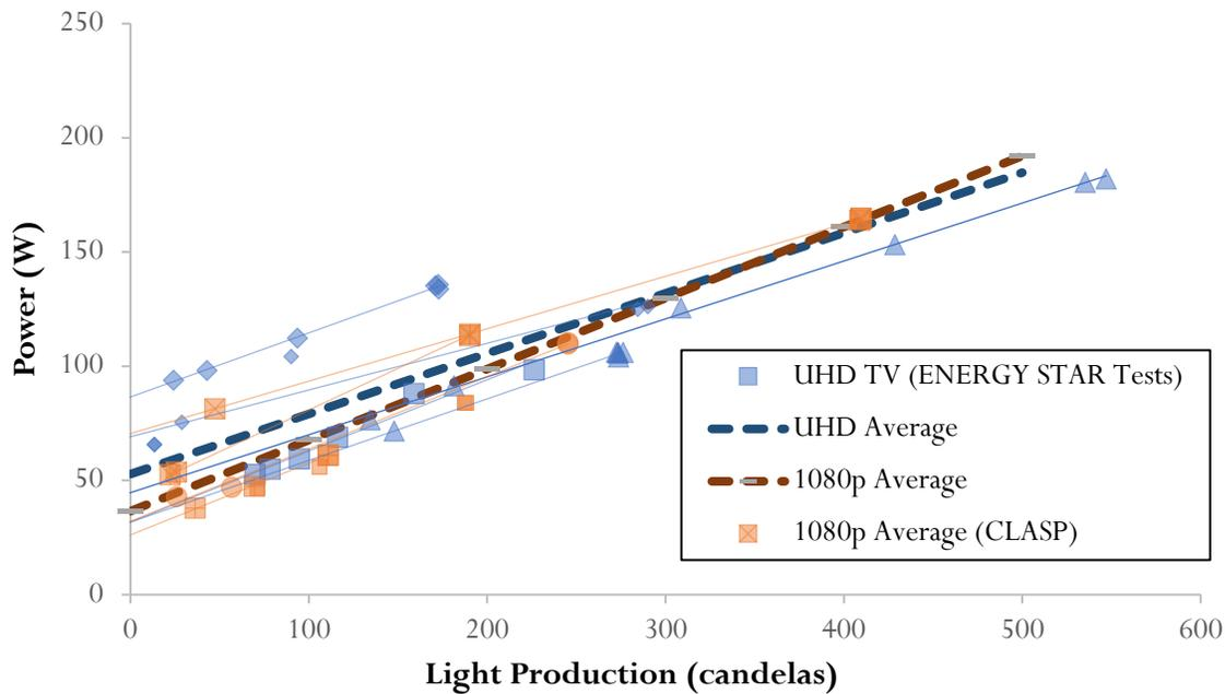
The slope for UHD TVs was found to be less than that of 1080p TVs. This is interpreted to mean that UHD TVs produced in 2015 or 2016 have more efficient backlights, or dimming techniques, than 1080p TVs produced in 2010 or 2011. However, the intercept for UHD TVs suggests an increased computing power (expected for higher resolution). The difference of the intercepts is about 16 W.
