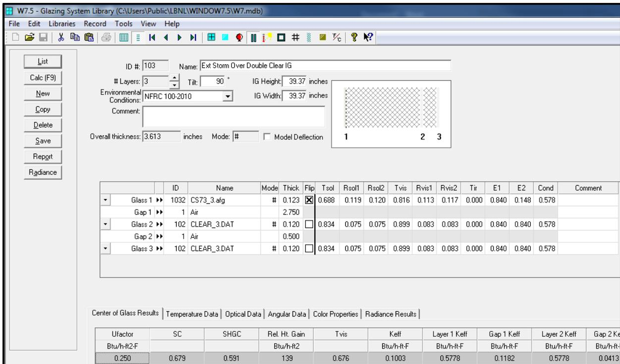
Figure 2: Center of Glass Properties for Existing Window with Double Clear Glass and Exterior Low-E Storm Window
