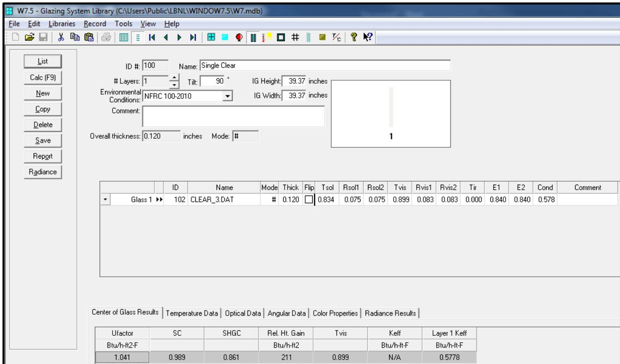
Figure 5: Center of Glass Properties for Existing Window with Single Clear Glass
