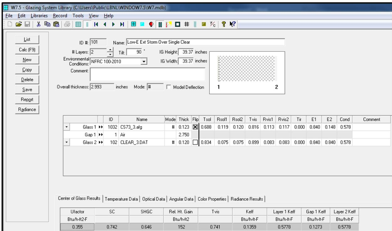
Figure 6: Center of Glass Properties for Existing Window with Single Clear Glass and Exterior Low-E Storm Window
