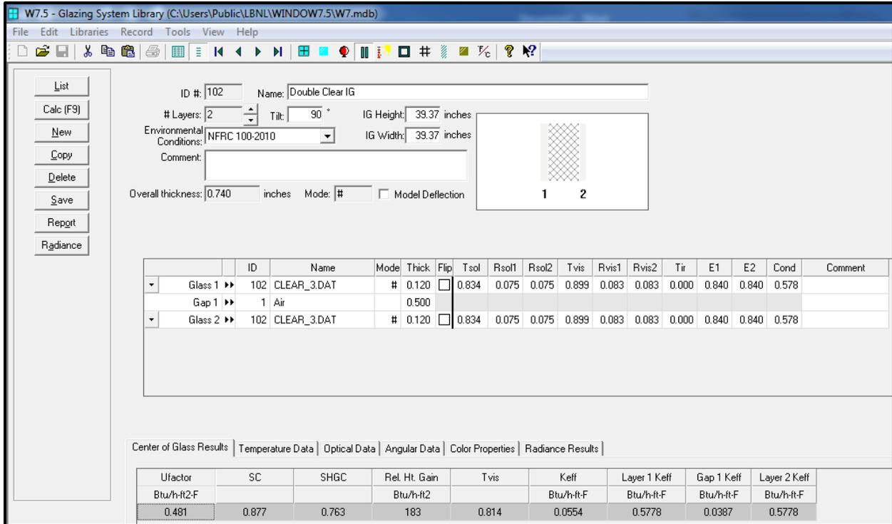
Figure 1: Center of Glass Properties for Existing Window with Double Clear Glass
