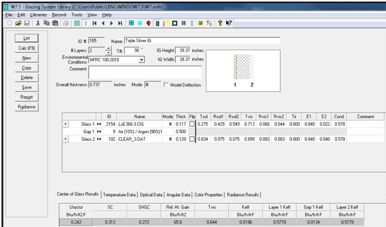
Figure 4: Center of Glass Properties for Replacement Window with Triple Silver Low-E IG
