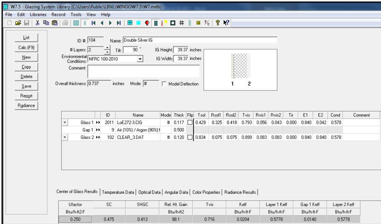
Figure 3: Center of Glass Properties for Replacement Window with Double Silver Low-E IG
