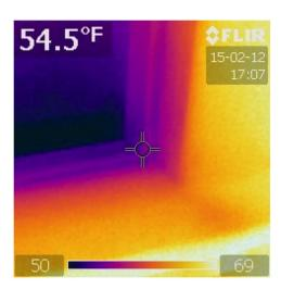
The photo on the left shows the surface temperatures of the inside surface of double pane windows without an acrylic interior storm window installed. The photo on the right shows a 23 degree warmer surface temperature of an acrylic interior storm window installed on the inside of the same double pane windows.
