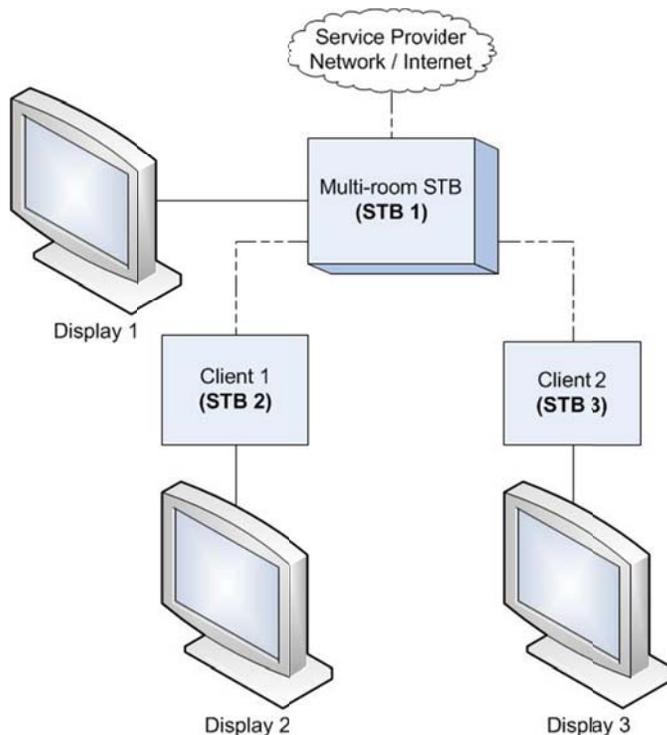
4.6.2 Multi-room STB Test Conduct: Multi-room STBs may be tested to measure the Client Only Power,  $P_{CLIENT\_ONLY}$ , and obtain the Client Only Incentive specified in Section 3.3.4, per the below requirements.
