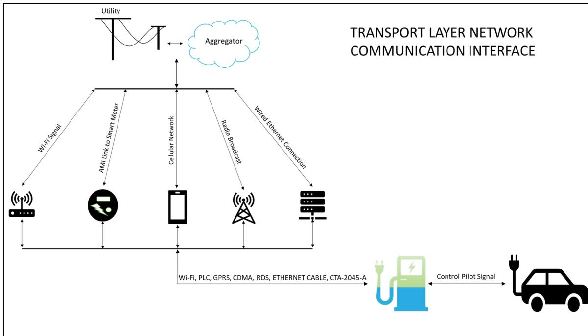
**Figure 2: EV Charging Infrastructure Network Communication Interface Options**
