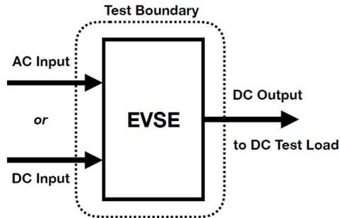
**Figure 2: Schematic of DC-Output EVSE Test Boundary**
