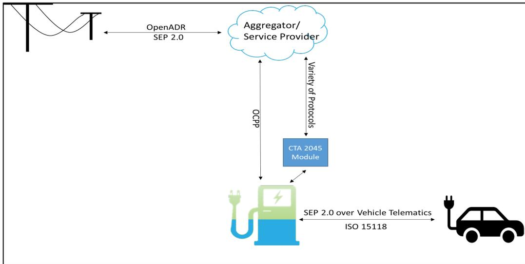
**Figure 1: Open Protocols based EV Charging Example Architecture**
