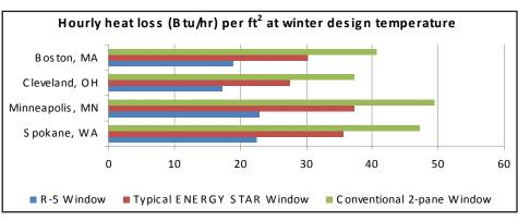
The rate of heat loss determines the window surface temperature and the need for perimeter heating.
