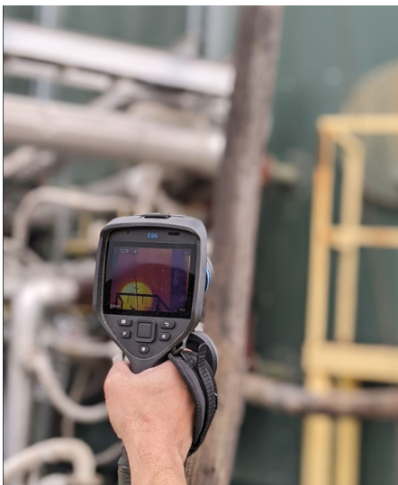
Figure 2. Thermal imaging gun showing a hot spot at the opening of a silo.
