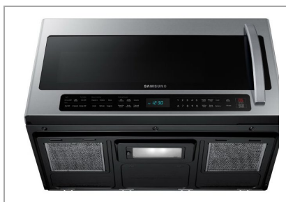
Figure 5: The bottom of this microwave has two airflow intakes. Some common airflow measuring devices may not be large enough to cover both ports, or the bottom surface of the microwave may not be flat, making accurate testing difficult.
