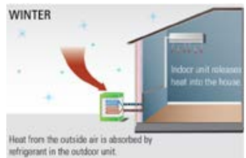
Figure 1. Ductless Mini Split Heat Pump Installed
