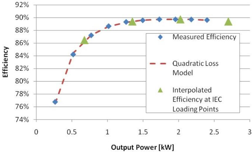
**Figure 4: Illustration of Efficiency Interpolation for Units Tested at Loading Points Other than Those Specified in IEC 62040-3.**
