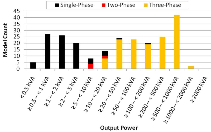
**Figure 1: Output Power and Number of Output Phases of Units Tested**
