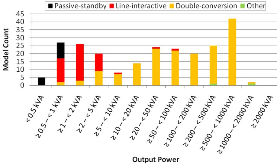
**Figure 2: Output Power and Topology of Units Tested**
