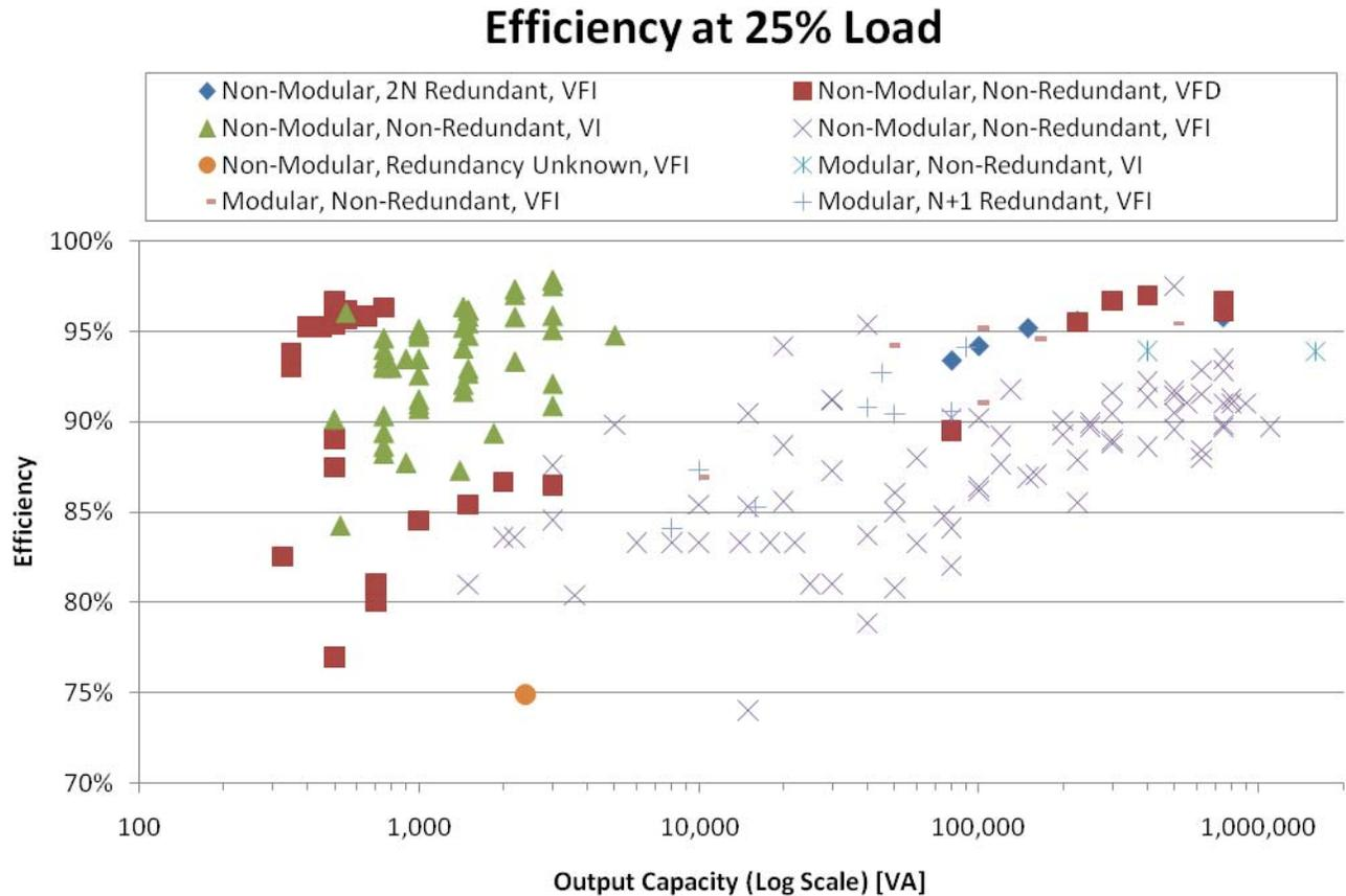
**Figure 6: Efficiency Test Results for Various UPS Configurations at 25% Load**
