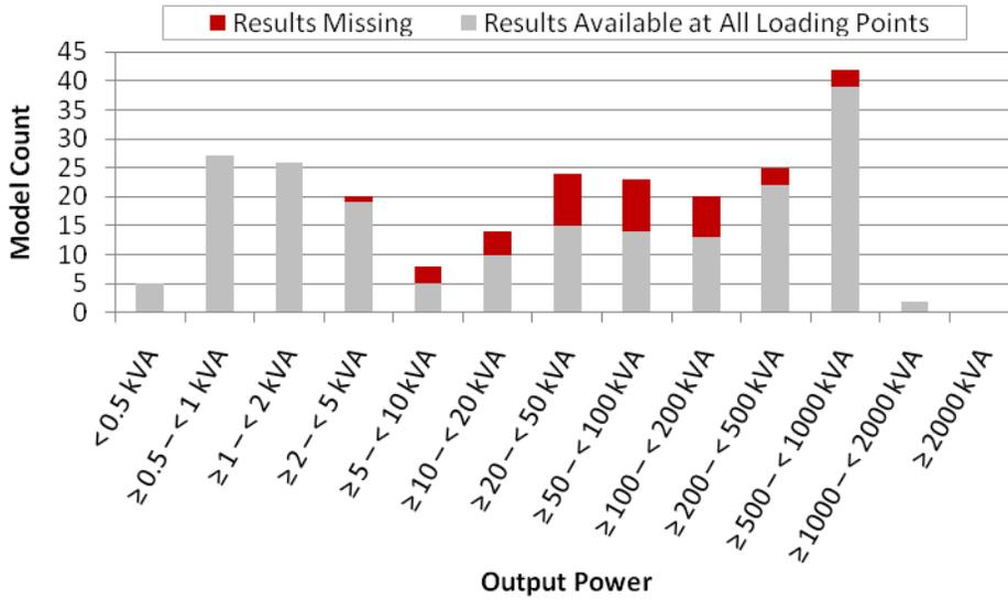
**Figure 5: Number of Tests with and without Results at All Four IEC 62040-3 Loading Points (100%, 75%, 50%, and 25% of Reference Test Load), Following Interpolation.**
