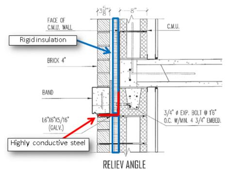
Figure 1: Wall construction utilizing shelf angle
