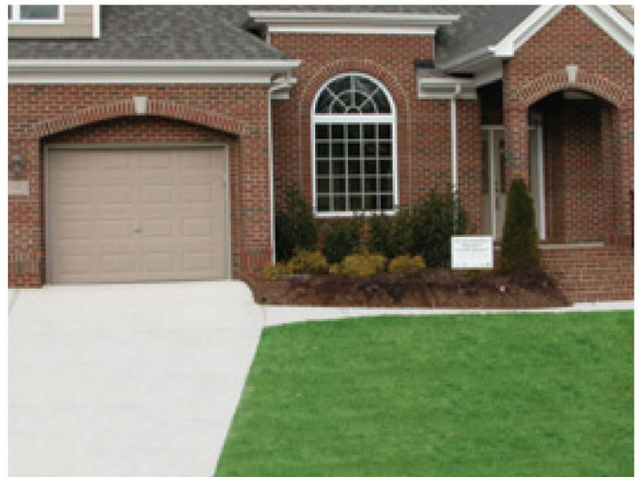
*The final grade slopes away from the house. Neglecting to consider exterior water management could lead to water damage.*
