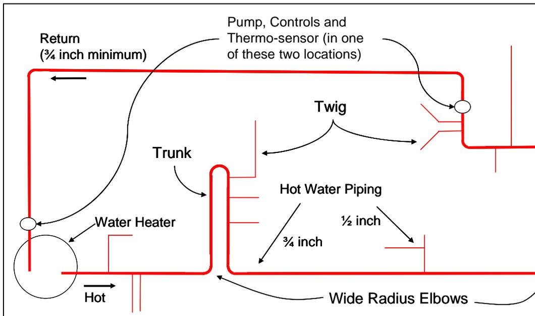
In a Structured Plumbing System layout, the on-demand pump is generally located on the return line near the water heater. In some cases it will be located under a sink in the hot water location furthest from the water heater, connecting the hot water supply line with the return line. Both of these options are shown in Figure 3. Sometimes the cold water line is used as the return as shown in the figure for single trunk and branch layouts.
