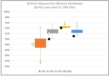
Based on this data and lacking clarity about whether the servers in the SpecPower database had 115v or 230v power supplies, we calculated savings for the average Internal Server as follows. The second row of the table shows our PSU savings assumptions by PSU load level relative to an 80 PLUS Platinum power supply at the lower end of the efficiency spectrum.
