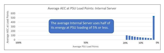
**Recommendation:** Revise power supply efficiency requirements to better represent real-world loading conditions, and to maximize the energy savings effect of PSU efficiency requirements.
