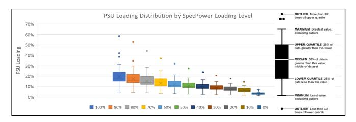
We then used the average PSU loading levels shown above to plot the average watts over time for these server classes:
