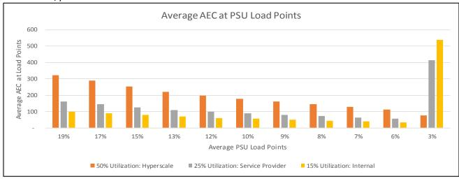
To better visualize how this distribution of energy relates to 80 PLUS test points, and to emphasize the importance of PSU efficiency at load levels, we then plotted the average energy distribution for Internal Servers (15% average system loading) with a PSU load level scale that spans 0% to 100%:
