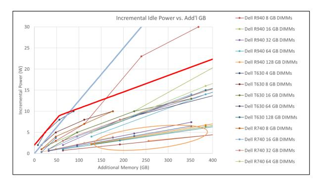
We have identified the most efficient cluster of configurations with the orange circle in the above chart. These lines have slopes of less than **0.033 W/GB**. These configurations have larger average DIMM module size then the less efficient configurations. And they tend to represent the latest server generation.<sup>4</sup>
