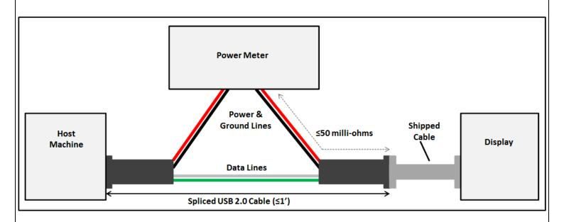
Figure 1: Example Spliced USB 2.0 Cable Arrangement
