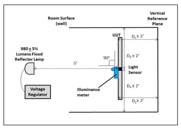
Figure 2: Test Setup - Top View
