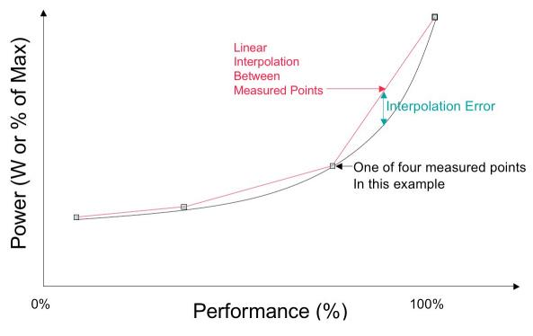
Figure A-1: Assessing measurement errors in the power plot data
