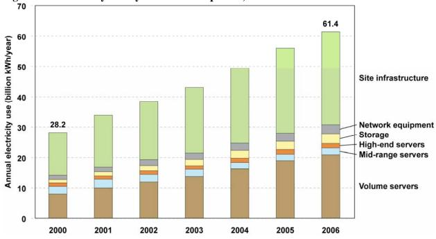
Figure 2-1. Electricity Use by End-Use Component, 2000 to 2006
